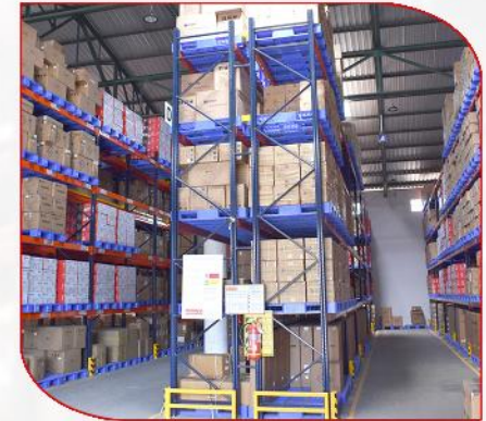
DOUBLE DEEP RACKS
